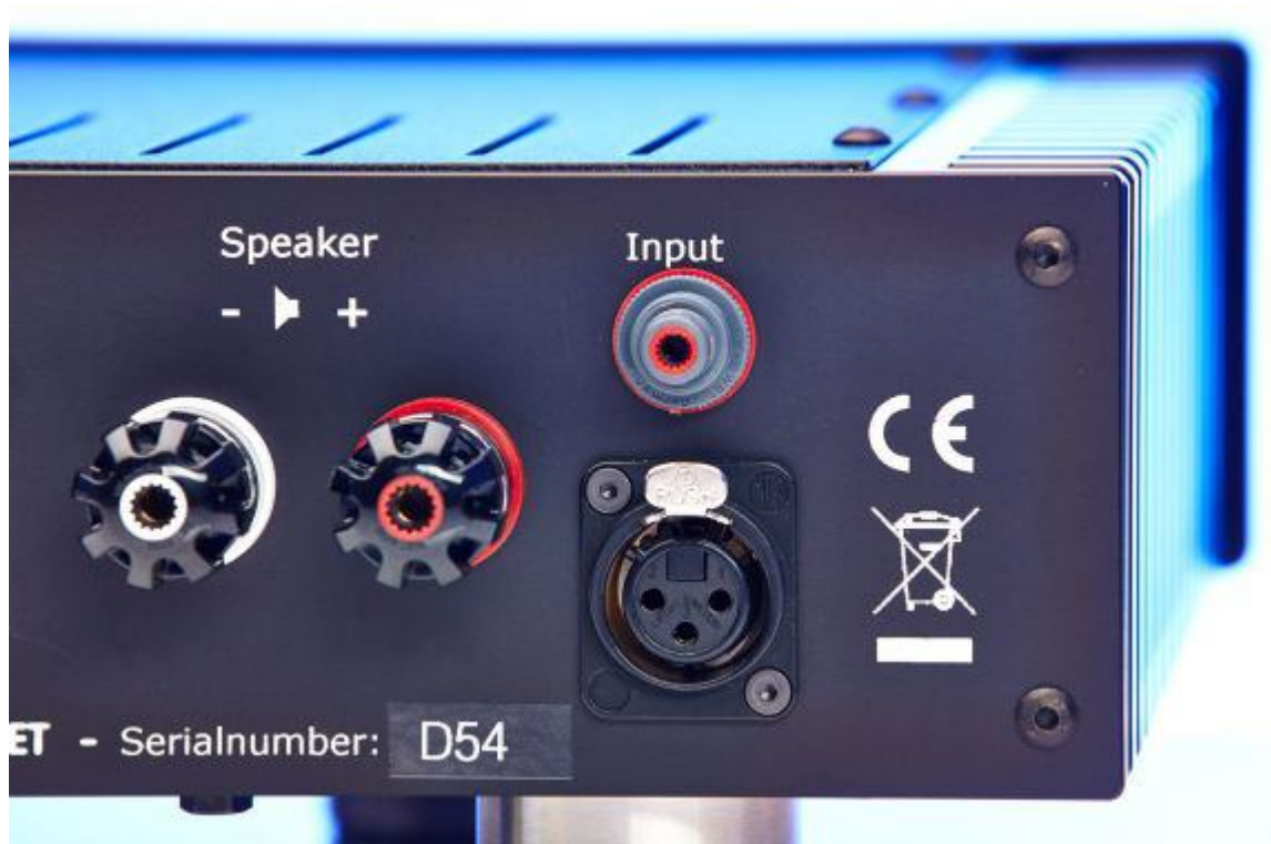
DETAILS TO IMPROVE THE SOUND: - VALVET A3.5 MKII COME EQUIPPED WBT AND WITH NEUTRIK (XLR)
